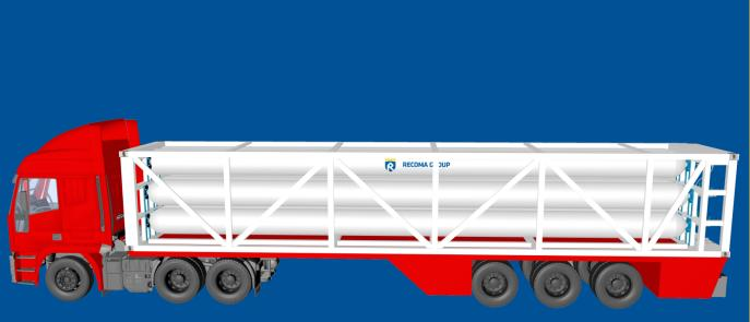
Road transportation is made by trailers that are equipped with 4 twist-lock. Safe and easy sea transportation is variable due to the stackability and 4 corner block structure of iso container.
